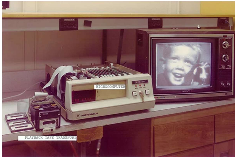
Figure 6. Additional equipment used to view images captured with Kodak's original digital imaging device. 39
