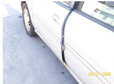
Figure 30. Photo #30: Seatbelt Stuck in Car Door
