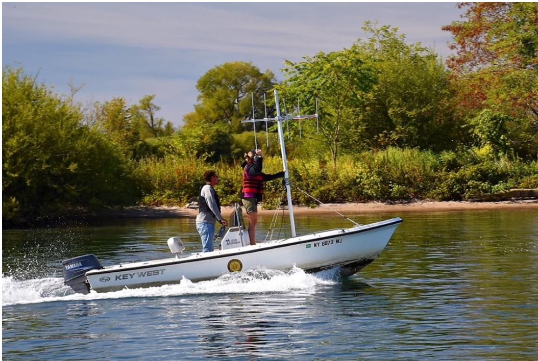
Figure 5. Six-element Yagi antenna used in active and passive radio telemetry.
