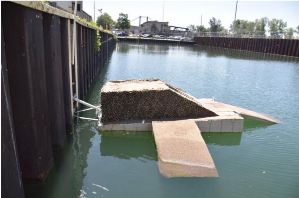
Figure 10. Basking/nesting platform deployed in the ACE and a hinge device that accommodated changing water levels.
