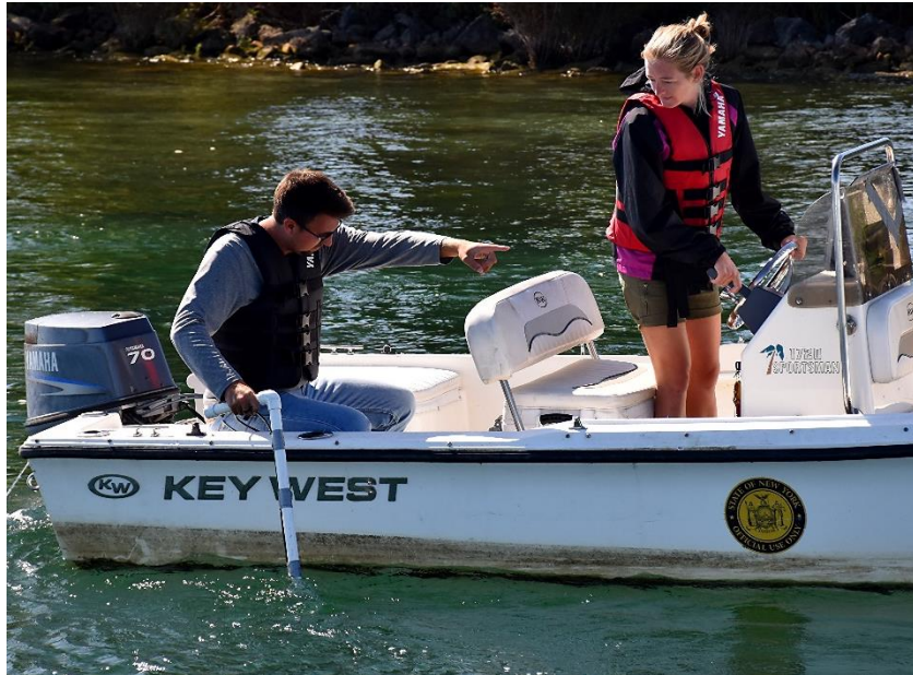
Figure 12. Active tracking using the six-element Yagi antenna, an H-antenna, and the Sonotronic sonic receiver.
