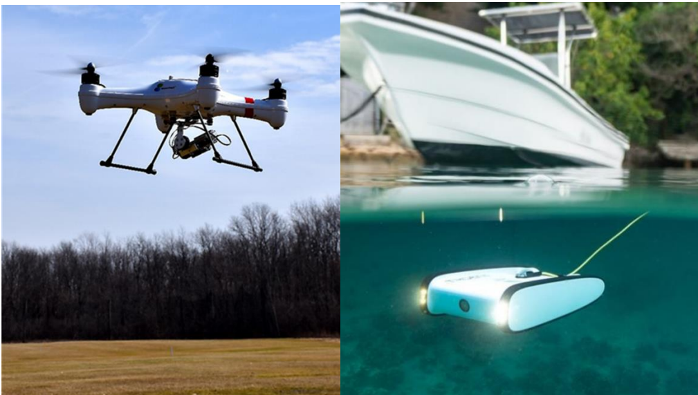
Figure 15. Left) Arial Splash Drone Waterproof with a mounted GoPro HERO4 silver. Right) OpenROV Trident underwater drone
