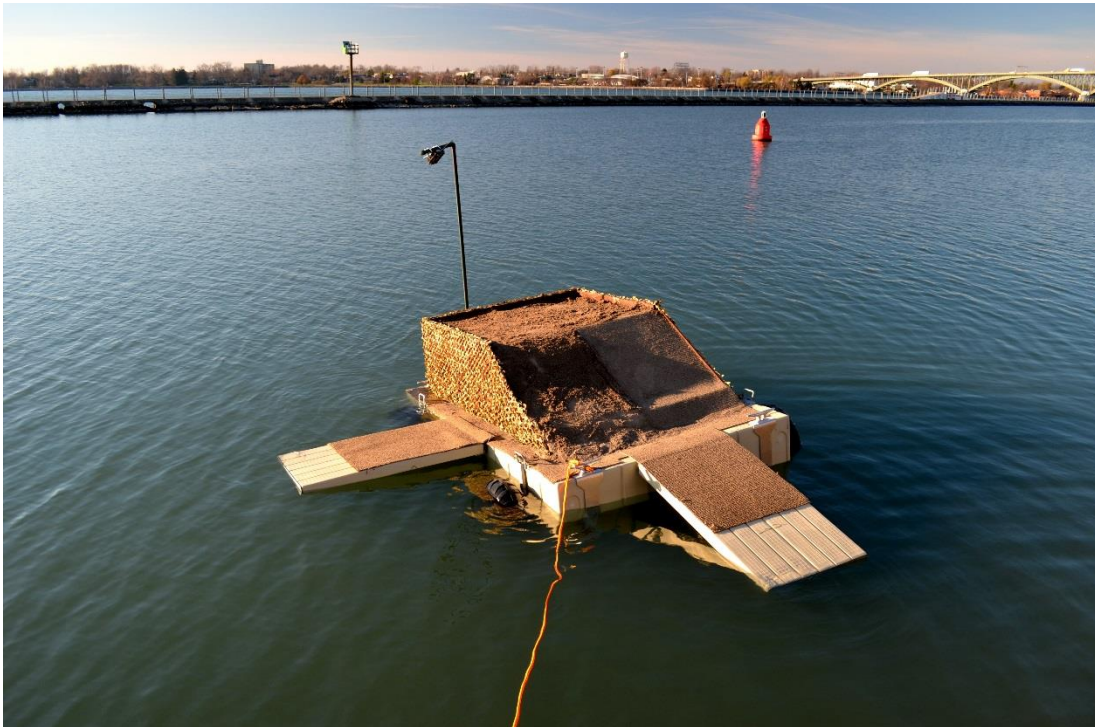
Figure 6. First completed platform with attached surveillance camera. This prototype was then modified to more evenly distribute the weight and had three ramps leading to the sand.
