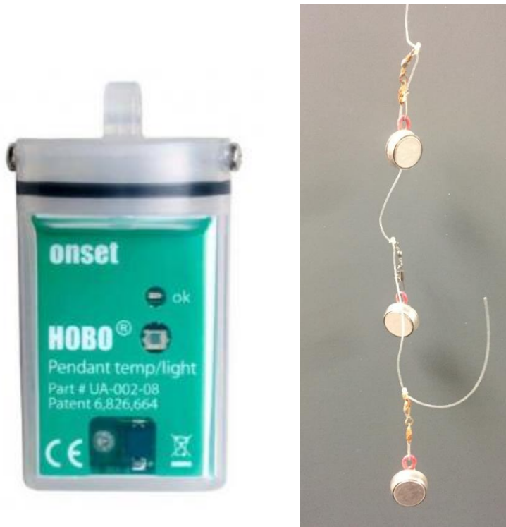
Figure 7. Left) HOBO data logger which recorded light intensity and temperature. Four were placed at each platform. Right) iButton data loggers recorded temperature, three of which were placed in the sand of each platform.
