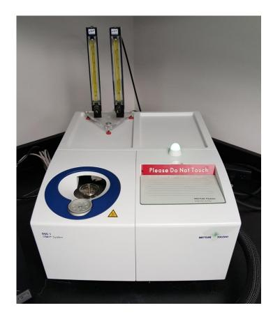
Figure 12: Image of a Mettler-Toledo DSC1.
