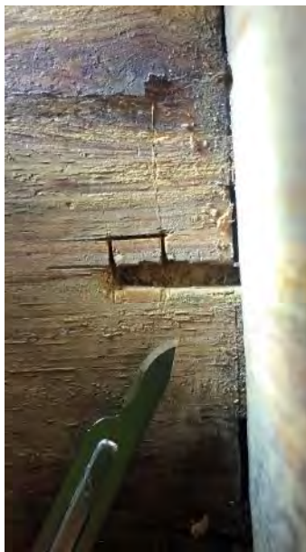
Fig. 12. Interior right back corner of cabinet, showing the sampling location for wood identification, above the lower runner mortise
