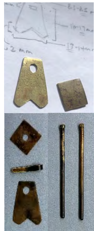
Fig. 18. Top: New brass pull-tab and decorative plate during fabrication, next to preparatory drawings and measurements. Bottom: Finished brass hardware.
