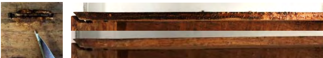
Fig. 14. Left: Adhesive reduction with a scalpel from an overfilled runner mortise. Right: before and after adhesive reduction on the bottom edge of the cabinet
