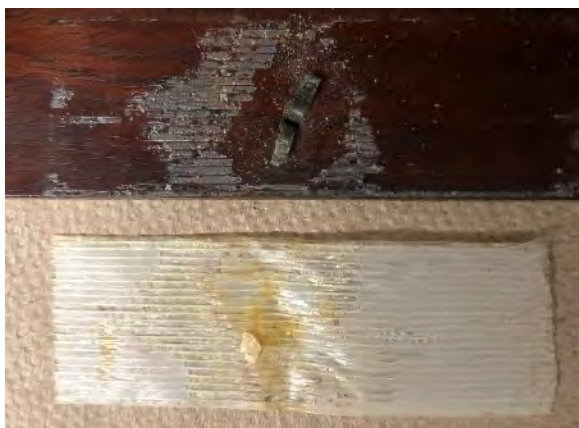
Fig. 17 - Tape removal from interior front wall of one of the small drawers. The brittle carrier has been removed, revealing the prongs and adhesive residue beneath.
