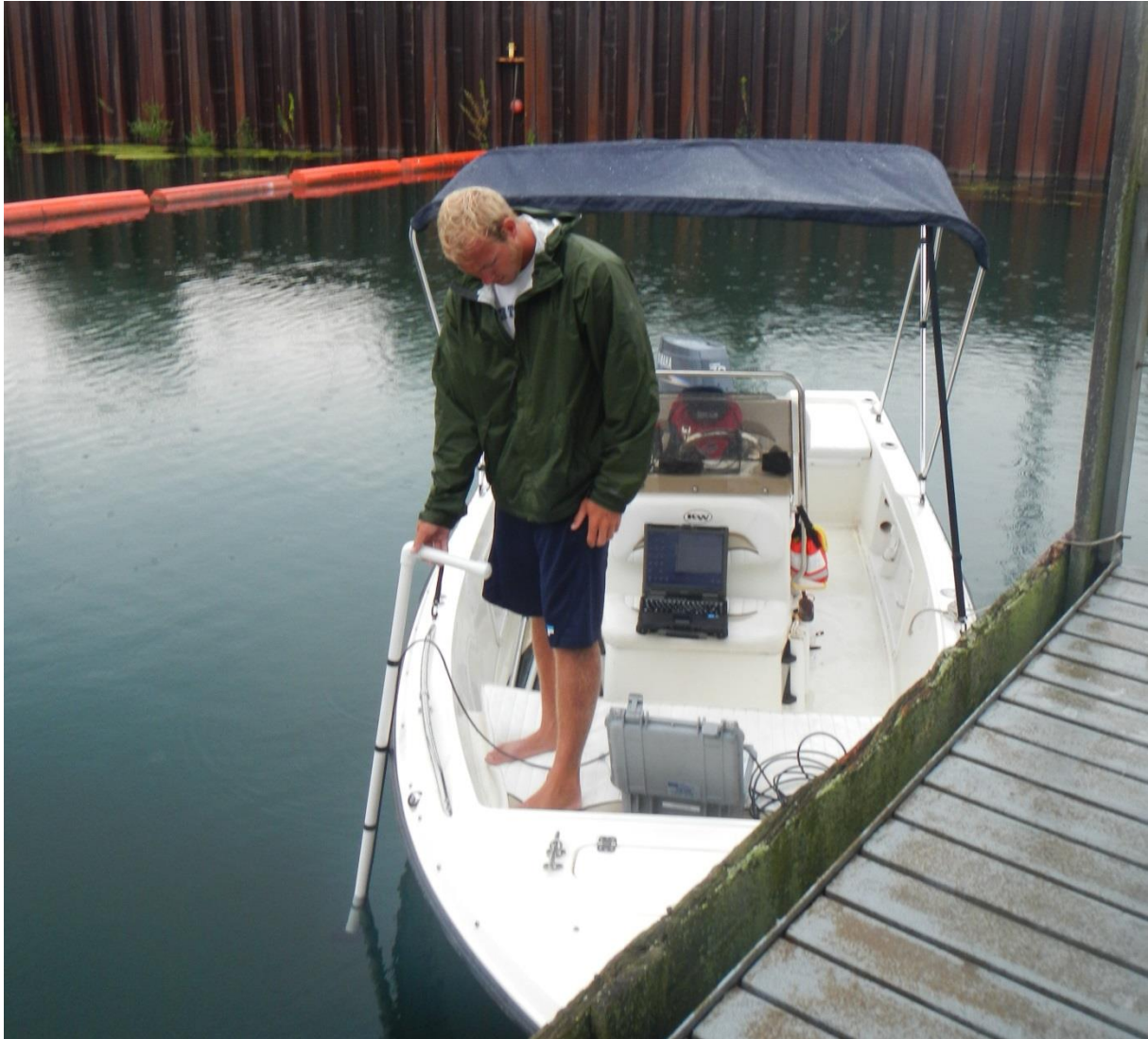
Figure 7. Active sonic tracking using the Vemco VH110 hydrophone connected to a Vemco VR100 topside receiver.
