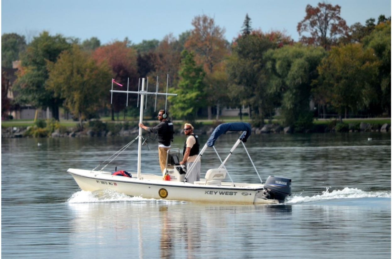
Figure 5. Active radio tracking using the boat mounted six-element Yagi antenna.
