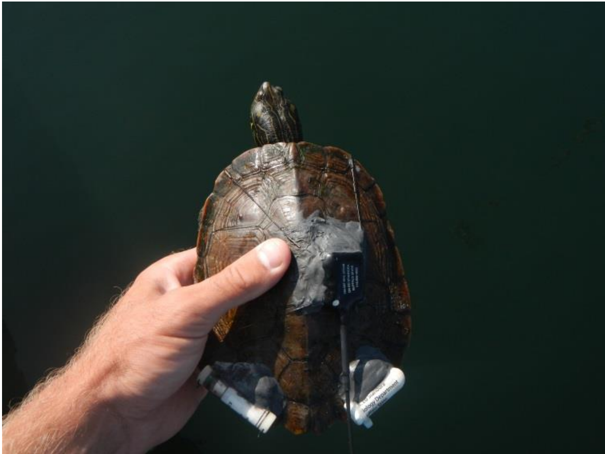
Figure 4. Female map turtle with attached instrumentation. Along keel of the carapace-radio transmitter, Posterior left-sonic transmitter, Posterior right-data logger.
