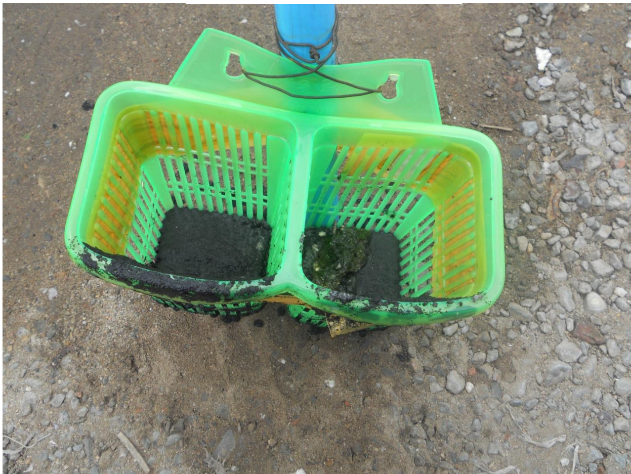
Figure 14. Modified sewer and wetland sampling apparatus.
