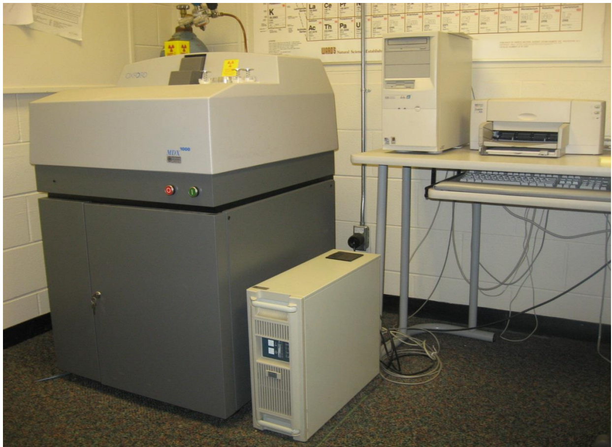
Figure 4. Laboratory-based Oxford instrument MDX1080+ MDXRF analyzer.
