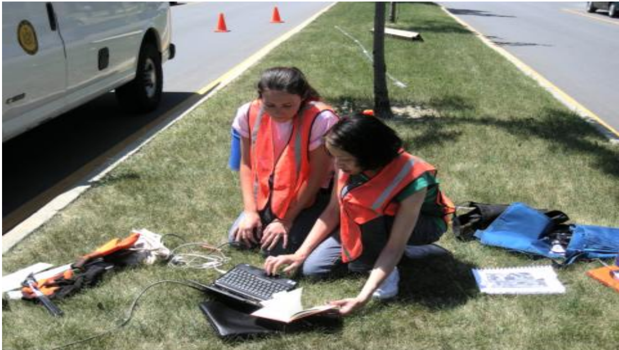
Figure 3.6: Downloading flow meter data. The flow meter was connected to the laptop using a communication cable to retrieve data.
