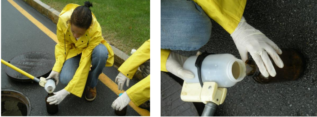
Figure 3.8: Transfer of sample. Attached bottled was transferred over to sample bottle until it was filled to 1000ml. While one student holds the nasco sampler the other student pours it into the sample bottle and another student preps the bottle.
