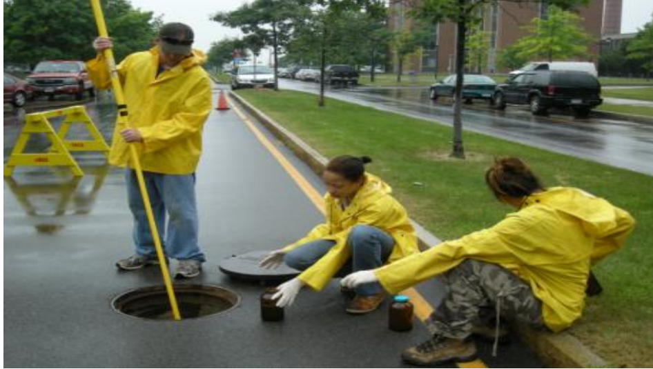
Figure 3.7: Wet weather sampling upstream at the inlet in manhole #230. A team of students assisted in collecting water samples for various time intervals. The 22 foot Nasco Sampler was used to collect the 15min interval sample for oil and grease on Rockwell Road.
