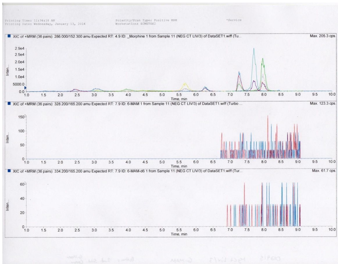
Figure 14. LC-MS/MS chromatographic peaks for the qualitative analysis of 6-MAM in the negative control 1:3 liver sample from the 012915 extraction. The top line displays all the components in the sample, the middle line displays 6-MAM in the sample, and the bottom line represents the 6-MAM internal standard that was added to the sample. The red and blue lines represent two transitions.
