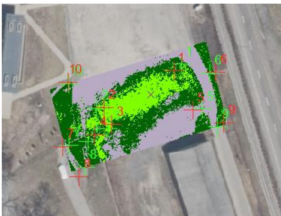
Figure 17 Georeferencing for the raster layer. Control points are indicated with numbered crosses. Red crosses are labeled on the base map. Green crosses are labeled on the classified image.
